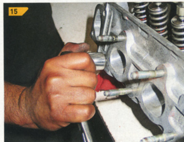
15 Ricky uses a stud tool to get the manifold studs completely threaded.
