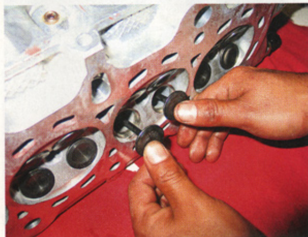
4 Then he slides in the intake and exhaust valves respectively.
