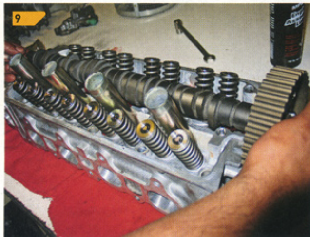
Now that the journals are good and lubed, Ricky drops the cam in.
