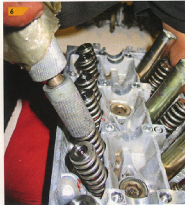
6 Like a true baller, Ortiz uses a proper keeper installation tool. We usually use a magnetic screwdriver and a spring compressor since we're poor.
