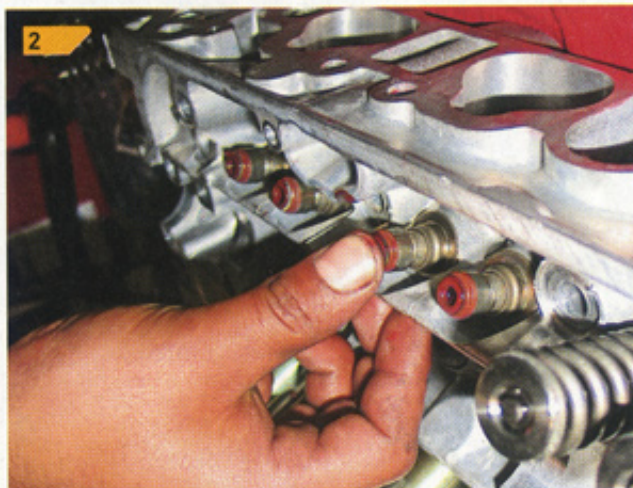
2 Ricky starts by pressing the valve seals on by hand.
