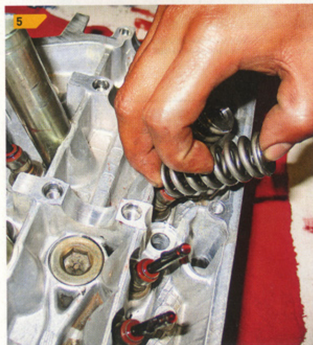
5 Using a foam pad to hold up the valves from beneath the combustion chamber, Ricky sets the valve springs and titanium retainers into place.
