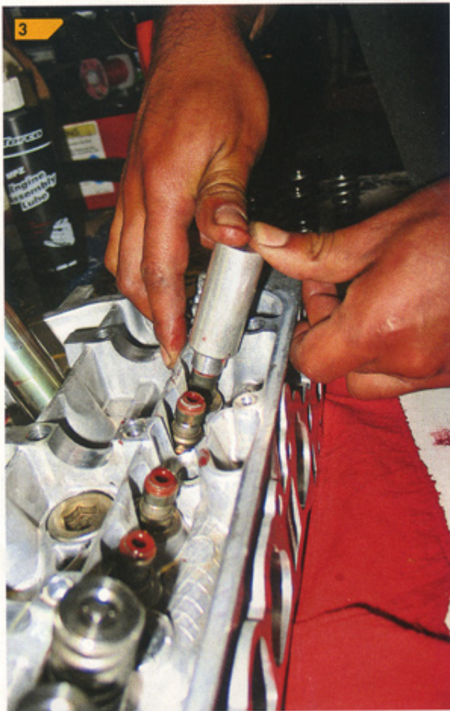
3 Once the seals are on snug by hand, Ortiz will use "Ricky's Special Tool" to press them on the rest of the way.
