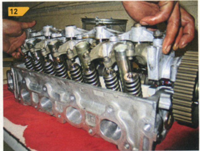
12 Ortiz drops the cam caps in place making sure not to take out the mounting bolts. Not only do these bolts hold the cam caps to the head, they keep the whole rocker assembly together.
