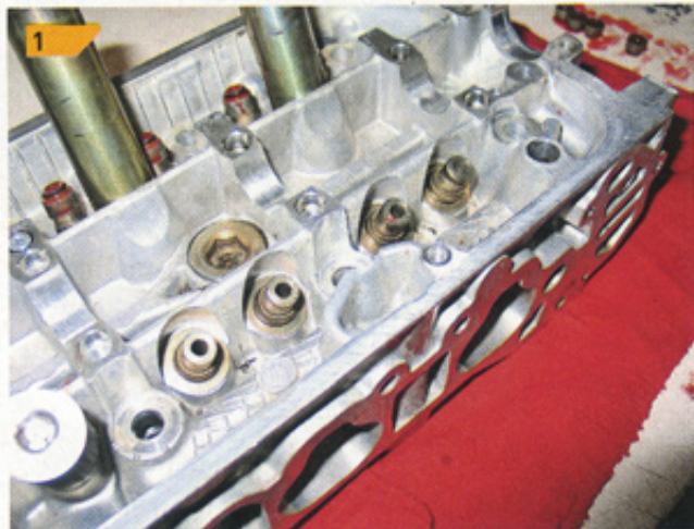
1 This is the head as we left it since the last installment. The porting is finished, but the head is still bare.
