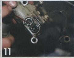
Brake cleaner is used to dislodge and dissolve any oil blowby that may have accumulated in the unit.
