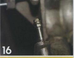
The fuel rail mounting studs from the stock manifold need to be removed and installed in the Skunk2 manifold, This method is the easiest way to remove stubborn studs.
