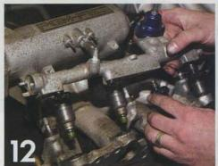
While the fuel rail won't be reused with the Skunk2 manifold, the RC Engineering fuel injectors will, so they must be removed from the stock unit.
