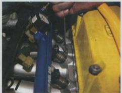
All of the nuts for the intake manifold are installed and tightened.
