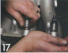
The RC Engineering fuel injectors are installed in the Skunk2 intake manifold.
