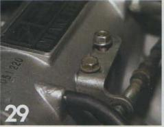
The bracket can now be bolted up to the plenum.
