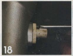
The stock air intake temperature sensor is installed in the Skunk2 manifold in the same location that it was in the stock unit.
