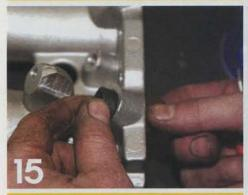
The rubber injector grommets from the stock manifold are installed in the Skunk2 manifold.
