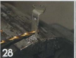
A slight modification to the throttle cable bracket must be made.
