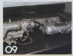
Here's a side-by-side comparison of the plenums on the two intake manifolds.
