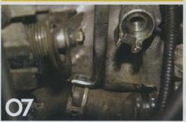
At the other end of the intake manifold, the coolant hose is removed.
