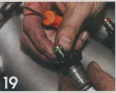
New injector O-rings came with the AEM fuel rail, and they are installed on the RC Engineering injectors.
