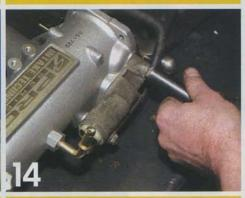
Next, the idle air control valve is bolted up to the Skunk2 intake manifold.
