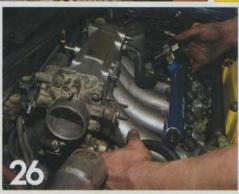
With the new gasket in place, the Skunk2 intake manifold can finally be installed onto the cylinder head.
