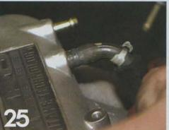
The vacuum hose for the breather system is hooked up to the plenum of the Skunk2 intake manifold.
