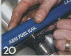
Now the fuel rail is installed on the injectors.
