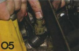
A small flat screwdriver is used to remove the clip and harness connector from the fuel injectors.
