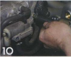
The idle air control valve is removed from the stock intake manifold.
