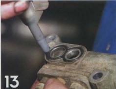
RTV sealant is applied to the mounting surface of the idle air control valve.
