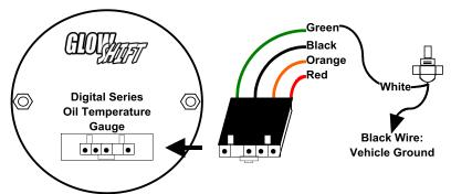
Wire Color Code Vehicle / Engine Ground (-) Black: Orange: 12v Headlamp (switched) Source (+) Red: 12v Ignition (switched) Source (+) Green: To **WHITE wire** on the Oil Temperature Sensor
