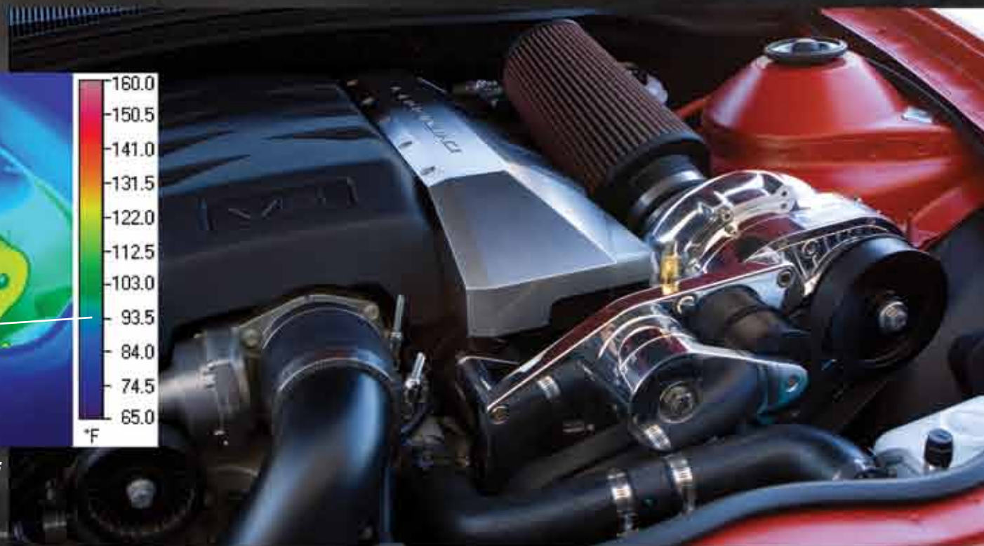
ProCharger with air-to-air intercooler, 8 psi
