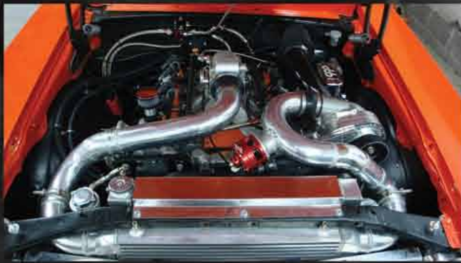
Customized ProCharger LSx Cog Drive Kit and aftermarket EFI system installed in a 1970 Chevrolet Nova.
