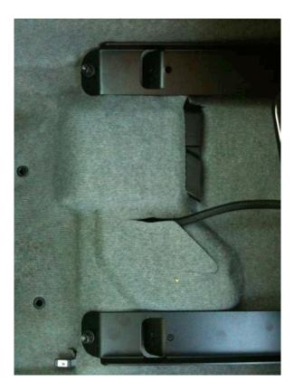
Step 8- Lay down the 2 black brackets inside your vehicle and line up the 4 hole locations. The parts look similar however the 90 degree bends on the brackets need to be facing the out. (see photo)
