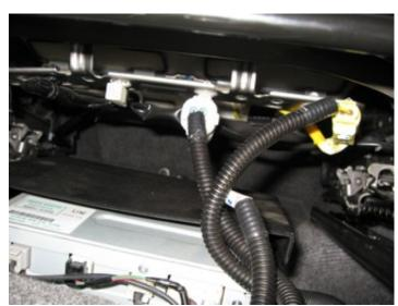
Step 4- (Optional Step. You do not have to unplug the cables) Unplug the 3 factory cables plugged into your car seat under the front portion of the seat. No tools required. Remember to plug these back in after you have completed the install.
