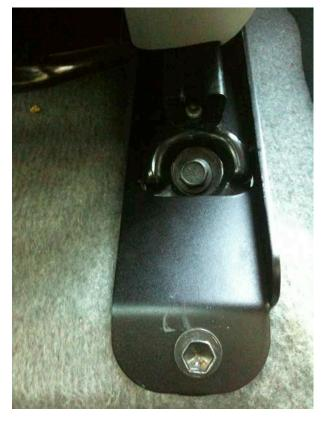
Step 9- Place the seat back into the vehicle. Line up seat front holes with EMS front holes. Finger tighten front 2 feet with provided black EMS bolts.
