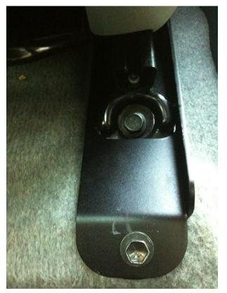
Step 9- Lay your factory seat on top of the EMS brackets and line up seat front holes with EMS front holes. Finger tighten front 2 feet with provided black EMS bolts.
