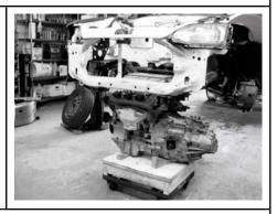
4 Once the engine is in the bay, move the engine towards the righthand bracket. Use the two 12mm x 35mm bolts with washers, the 12mm x 120mm bolt, 12mm nut and two more washers and attach the right-hand mount to the bracket and the engine using the hardware from the right-hand mount hardware bag. Leave all the bolts finger tight at this time.
