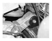
10. Torque all mount and bracket bolts according to specifications below. (14mm, 17mm, 19mm Socket & 17mm, 19mm Wrench)
