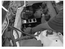
5. The left-hand should be installed using the left-hand mount hardware. Use the original Honda bolt to attach the mount to the car. On the two longer bolts used to attach the mount to the transmission bracket, a washer is used only on the top of the bolt. No washer is used on the underside of the bracket. All the other bolts use a washer on both sides of the bolt.
