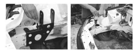
7. Slide the bracket back on the frame rail and thread the two bolts down through the bracket and out the bottom. Tighten the bolts to about 10ft/lbs of torque. Be careful to check the alignment of the bracket so the bolts thread easily all the way through the bracket. Do not over tighten.
