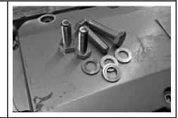
12 Using the longer bolts at the rear and the shorter bolts at the front, bolt the mount on the rear subframe in the same location as the stock rear mount. Just finger tighten the bolts at this time.
