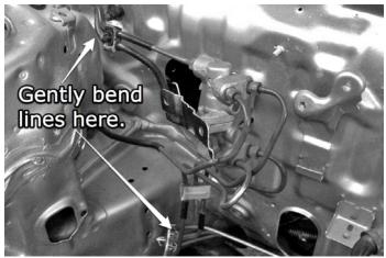
Next flip the bracket on the prop valve so it can be used to mount it to the firewall. You'll need these tools; C-clamp with a 4" opening and T-30 Torx Security Bit. Use the C-clamp to hold the prop valve together and unscrew the two T-30 Torx screws holding the bracket on. Flip the bracket towards the firewall as shown in the picture and retighten the screws.
