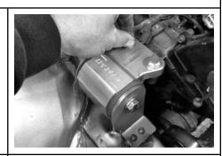
You will need the 12mm x 60mm and 12mm x 30mm bolts to install the left-hand bracket
