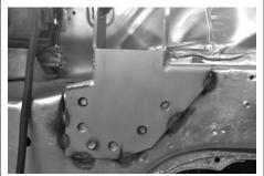
Next trim the right-hand headlamp sheet metal to clear the front cylinder head valve cover. About and inch of sheet metal needs to be trimmed from the car so the valve cover won't interfere once the engine is bolted in place. You may want to trim a small amount and try the engine in for clearance. More can be trimmed if needed. If you plan to mount the stock alternator in the stock location more will need to be trimmed.
