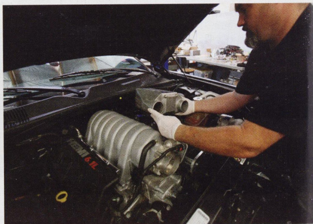
> The aftercooler has two tabs that locate it on the fuel rail but is otherwise held in place with the inlet and outlet tubing.
