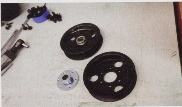
> The kit also comes with a new power steering pulley. The stock pulleys have had issues with cracking, and since the supercharger's power draw puts more stress on the accessory drive system, Vortech includes a new, stronger power steering pulley to replace the weak stocker.
