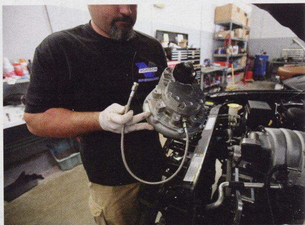
> The V-3 head unit has a fully self-contained oiling system. This is the drain hose that allows you to drain the oil for servicing (rarely needed) without having to remove the blower.
