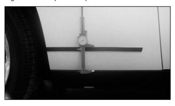
7.) Mark a line on the tape 12" in front of the wheel well as shown below.
