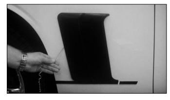
12.) Once all of the liners are removed apply firm pressure along the perimeter of the quarter scoop to secure it to the vehicle as shown below.
