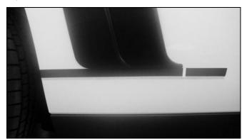
9.) Once quarter scoop is properly aligned gently pull the outer lining tab to the rear upper corner of the quarter scoop as shown below. Apply light pressure where the tape has been exposed. Be sure quarter scoop remains aligned as you pull the tape linings.
