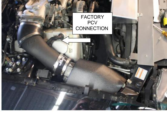
Go back and make any adjustments to the tube and tighten the clamps. Installation is complete.
