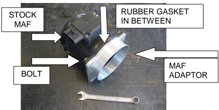
Install the filter onto the MAF adaptor and the silicone reducer onto the MAF. Next install Throttle body coupler onto 4 JLT tube, then the tube into silicone reducer making a complete unit from throttle body to filter.
