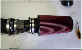
**5** PULL the Inlet Air Temperature sensor from your stock inlet and install in the grommet on bottom side of JLT tube.
