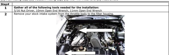
Pull the thin, hard vacuum line out of the large connection on the stock intake tube
