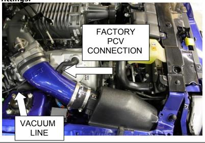
Go back and make any adjustments to the tube and tighten the clamps (ONLY FINGER TIGHT). Installation is complete.
