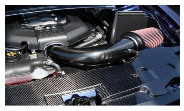
This kit includes an S&B Powerstack pre-oiled reusable air filter. The frequency you should clean your filter will depend on your driving conditions. It is recommended to check your filter at every oil change or 3,000 miles. If there is a build up of dirt as thick as the wire mesh, then it's time to clean your filter. As dirt builds up on your filter, the restriction of the airflow also increases. More frequent cleanings will improve your fuel economy and your vehicle's performance.
