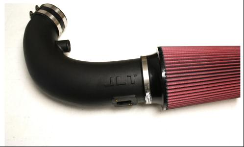
Install the coupler end on the throttle body and rotate down to sit in the heat shield and tighten clamps. The tube will sit on the heat shield gasket and the rubber end of the filter will rest on the apron panel.
