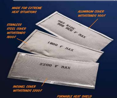
More than just another heat shield, Inferno Shields™ can be custom configured to handle whatever your thermal requirements may be. These heat shields can be bent, folded, and twisted to form a custom shape. Our heat shields come in three different grades of alloy: aluminum (900°F continuous), stainless steel (1800°F continuous) and Inconel (2200°F continuous). All of these alloy heat shields have an inner ceramic pad that can be trimmed for a custom fit.
