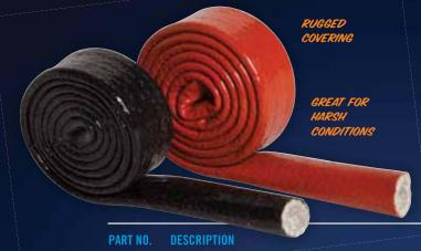
The rugged silicone covering makes it resistant to chemicals, non combustible, abrasion resistant, and fraying is also reduced to a minimum. This rugged covering makes HP Fire Armor™ ideal for welding lines and cables. You can also use HP Fire Armor™ for brake lines, fuel lines, wiring harnesses, and cables. HP Fire Armor Sleeving™ withstands 450°F continuous and works great for areas where harsh environments exist that require heat shield insulation.
