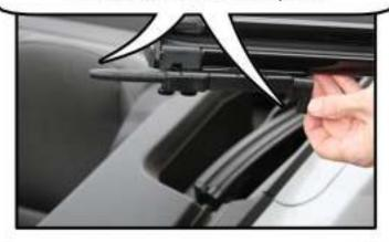
Now lower the wind deflector into the back seat area so the rear bracket goes into the slot beside the rear seat.
