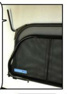
Then extend the barrel bolt on the passenger side as well. And turn the handle down to lock it in place.
