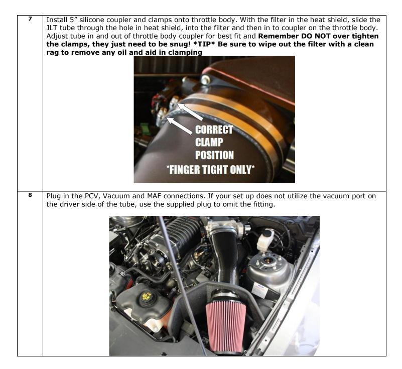
This kit includes an 5x9" S&B Powerstack pre-oiled reusable air filter. The frequency you should clean your filter will depend on your driving conditions. It is recommended to check your filter at every oil change or 3,000 miles. If there is a build up of dirt as thick as the wire mesh, then it's time to clean your filter. As dirt builds up on your filter, the restriction of the airflow also increases. More frequent cleanings will improve your fuel economy and your vehicle's performance.
