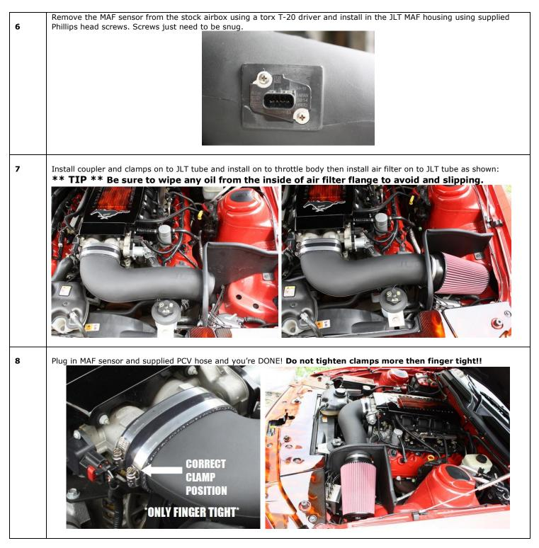
This kit includes an S&B Powerstack pre-oiled reusable air filter. The frequency you should clean your filter will depend on your driving conditions. It is recommended to check your filter at every oil change or 3,000 miles. If there is a build up of dirt as thick as the wire mesh, then it's time to clean your filter. As dirt builds up on your filter, the restriction of the airflow also increases. More frequent cleanings will improve your fuel economy and your vehicle's performance.
