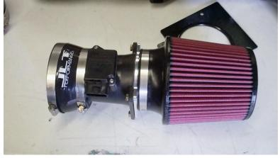
Install silicone coupler and clamps on to the JLT tube, then insert round end into the hole in the apron plate and rotate it down and on to the throttle body. Tighten the clamp at the throttle body and leave the clamp on the tube loose for final adjustment.
