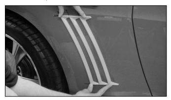
**8.)** Once quarter molding is properly aligned, remove the top lining by pulling the top tab toward the front of the vehicle as shown below. Be sure that Quarter Molding remains properly aligned as you pull the tab. Apply firm pressure where lining has been removed.
