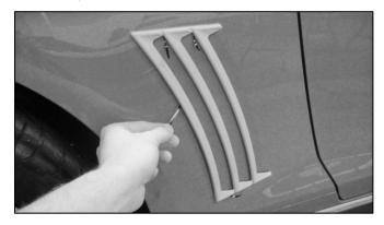
**10.)** Remove the bottom lining by pulling the bottom tab toward the front of the vehicle as shown below. Apply firm pressure where the lining has been removed.
