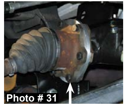
Passenger side shown with one 15/16" C.V. spacer.
