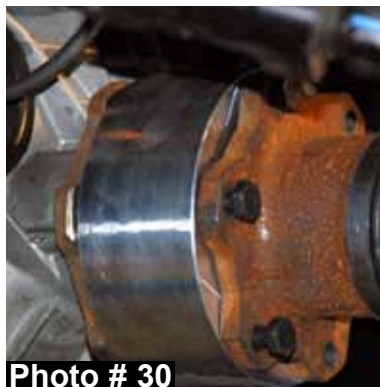
Driver side shown with 3.35" cv-shaft spacer.
