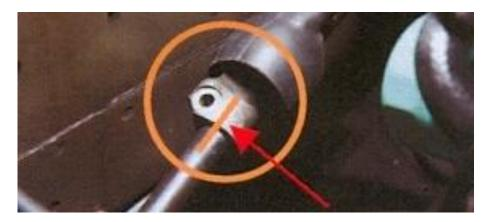
3. Loosen the bolts on the subframe. DO NOT REMOVE THE BOLTS. Drop the subframe 8mm from the chassis of the vehicle.
