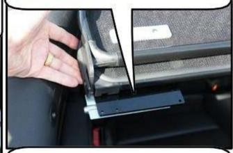
THEN SLIDE THE BARREL BOLT INTO THE HOLE AND TURN THE BOLT TOWARDS THE FRONT OF THE CAR AND PUSH BACK TO LOCK IT INTO THE LOCKED POSITION. ONCE YOU HAVE BOTH BARREL BOLTS LOCKED INTO PLACE YOU ARE DONE.
