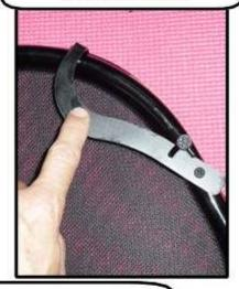
THE WIND DEFLECTOR WILL FIT IN YOUR TRUNK WHEN NOT IS USE. IT IS A TIGHT FIT. START BY PUTTING THE SIDE WITH THE BARREL BOLTS IN FIRST. PLACE ONE IT INTO THE FAR CORNER OF THE TRUNK.
