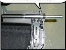
THEN EXTEND BOTH OF THE REAR BRACKETS AND TIGHTEN THE THUMB SCREWS FINGER TIGHT.
