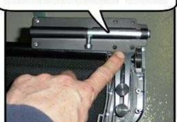
NEXT SLIDE THE BARREL BOLT DOWN AND INSERT THE TWO THUMB SCREWS INTO THE TOP TWO HOLES.
