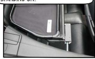
THEN LOWER THE WIND DEFLECTOR SO IT IS FLAT AND INTO REAR SEAT AREA. THE REAR BRACKETS WILL SIT ON THE LIP THAT IS BELOW THE LID THAT COVERS YOUR CONVERTIBLE TOP. YOU MAY NEED TO ADJUST THE REAR BRACKETS SLIGHTLY INWARD TO FIT YOUR BMW AS EACH CAR IS A LITTLE BIT DIFFERENT.
