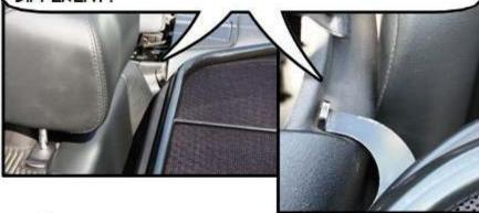
NOW ON THE DRIVERS SIDE, WHILE STILL HOLDING ON TO THE WIND DEFLECTOR, LOWER IT SO THE BARREL BOLT IS IN LINE WITH THE HOLE IN THE TRIM PANEL.
