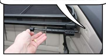
Next reach back and slide the back bolt into the rear hole and turn the handle down to lock the barrel bolt.
