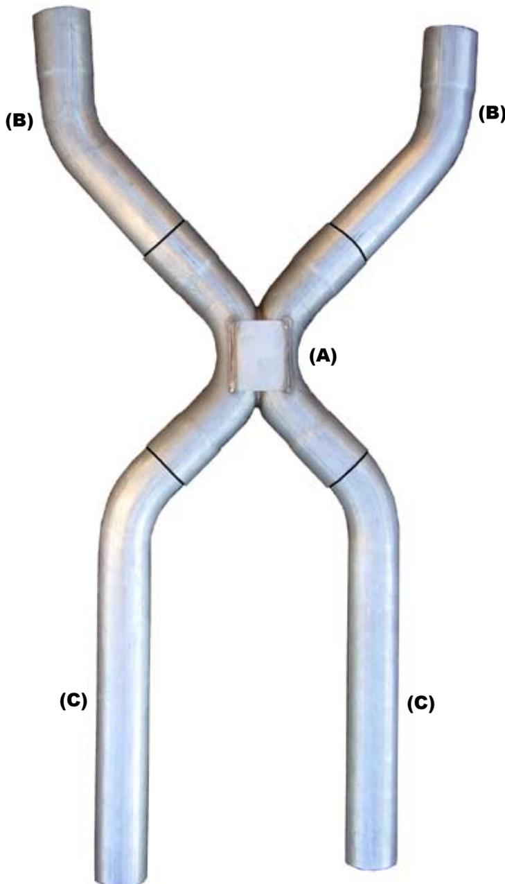
1. This five piece kit is a universal kit produced to fit many applications. Measuring and cutting will be required. The x-pipe is designed to connect to your collector reducers or down-pipes under the transmission cross-member.
