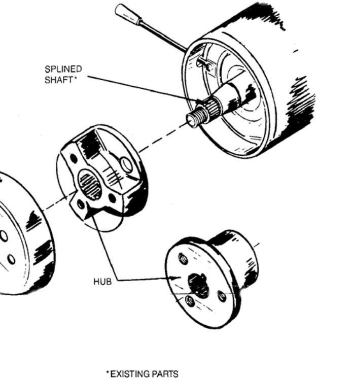
6. Position post cover (unless kit has a black coated hub, in which case a cover is not provided), wheel and retainer onto hub using the three hex bolts provided. Tighten these bolts to 10-12 ft/lbs. Note that excessive torque will result in damage to the hub. The wheel retainer nut, if properly tightened, will firmly hold the wheel/hub assembly onto shaft.
