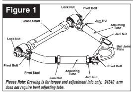
SPC Performance Pro Series **Part No.** 94340 - ADJUSTABLE UPPER CONTROL ARM. The arm accepts the standard SPC **Performance Ball Joint - Part No 94006** or Moog K5208, or equivalent, bolt in style ball joint.
