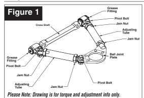
SPC Performance Pro Series Part No. 94332 Right & Left - ADJUSTABLE UPPER CONTROL ARM. The arm accepts the standard SPC Performance Ball Joint - Part No 94006 or Moog K5208, or equivalent, bolt in style ball joint.
