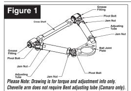
SPC Performance Pro Series Part No. 94330 (Right Side) or Part No. 94331 (Left Side) -ADJUSTABLE UPPER CONTROL ARM. The arm accepts the standard SPC Performance Ball Joint - Part No 94006 or Moog K5208, or equivalent, bolt in style ball joint.
