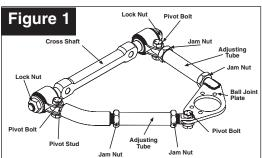
Please Note: Drawing is for torque and adjustment info only. Chevelle arm does not require Bent adjusting tube (Camaro only). 94324 includes 20 degree angled ball joint plate.
