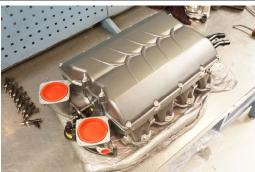
70 Locate the heat shield in the install kit and fold upwards along the creased lines to a 45° angle as shown
