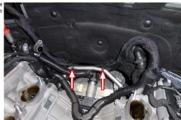
38 Remove the plastic insert from the panel, and route the harness through panel relief as shown.
