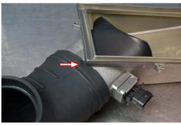
154Fit the factory intake boot clamps to secure the ducts to the air box lids, once tensioned the clamp should just sit below the edge of the air box lids corner as shown.
