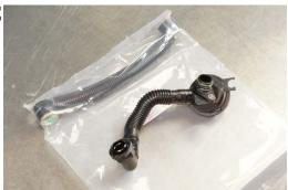
58 Slice into the hose to release each fitting as shown. Take care not to cut too deep as there are orings.
