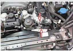
22 Remove the T30 fastener securing the power steering reservoir to the front engine lift bracket.
