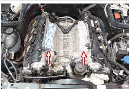
32 Compressing each sideclip of the connector, disconnect the PCV valve hose from the engine.
