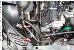
120 Connect the coolant pump \trigger wire extension and route towards the engine-bay fuse box (beside the brake booster).
