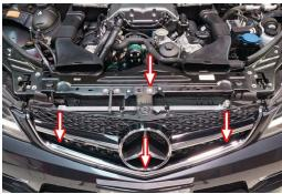
162 Reinstall the radiator support panel cover in reverse order of removal, making sure all retaining clips have securely seated.
