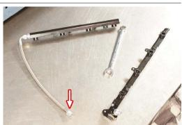
84 After ensuring they are free from any debris or damage, install the clean fuel injectors into the rail.
