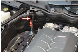
80 Using the supplied fuel emission hose, install and clamp onto the remaining manifold port as shown.
