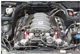
14 Disconnect the brake booster tube from the back of the manifold at the shown location by squeezing the retainer tabs while extracting the white connector.
