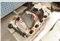
48 Undo the thirteen (13) T30 fasteners securing the lower manifold to the upper section.
