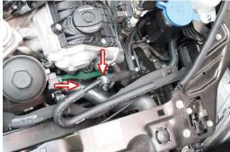
108 Remove the hose joiner from the purge solenoid (vertical arrow).
