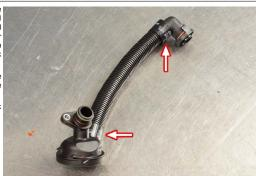
60 Install the upgraded PCV valve assembly onto engine.
