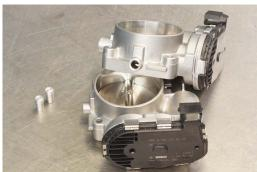
54 Using a soft mallet, gently but firmly tap in the plugs until they are firmly seated into the throttle body vacuum ports. A smear of Loctite or similar sealer may be used, but is not mandatory.
