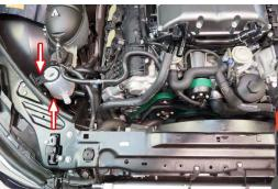
144 With the supplied clamps, fit the reservoir to LTR hose as shown.
