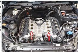
76 With assistance, lower the supercharger into position over the manifold studs making sure that all looms and harnesses are clear.
