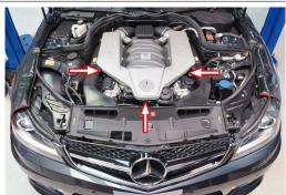
4 Remove both intake ducts by pulling back on the duct at the air box and unclipping from the front trim panel.
