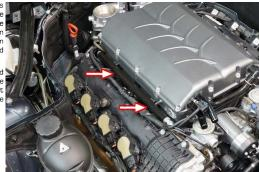
90 Reusing the factory fuel pressure sensor and supplied fasteners, install the sensor into the rail manifold and connect the electrical connector.
