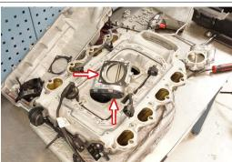
52 Remove the MAP sensor, manifold runner activation solenoid, and the short vacuum hose shown. These items will be reused during the install.
