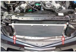
134 Install the two (2) top LTR brackets by using the supplied pop rivets to secure the brackets to the LTR as shown.
