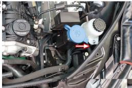
106 Remount the washer bottle support bracket to the washer bottle and include the power steering reservoir bracket, fastened to the radiator support panel with the original fastener.
