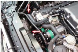
142 With the hose installed, make final orientation adjustments of the pump position and then complete torqueing the clamp fastener.
