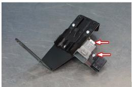
116 To mount the degas reservoir bracket, the rear most lower brace fastener will need to be removed (vertical arrow).
