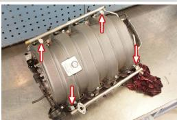
46 Remove the all the injectors from the rail by gently prying off the injector retaining clips and pulling the injectors out of the rail.
