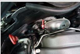
28 Remove the cable ties securing the injector harness to the fuel rail and proceed to disconnect each of the injector plugs from the injectors.
