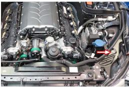
98 Unclip and remove the washer reservoir support bracket, this will be reinstalled at a later stage.
