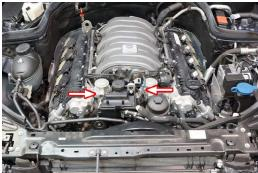
20 Using a suction tool, remove as much power steering fluid as possible from the reservoir.
