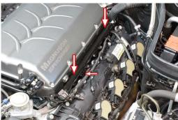
86 Once seated, using the supplied fasteners carefully secure the fuel rail to the supercharger.
