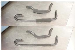
102 Install and clamp the new power steering feed hose to the new power steering reservoir as shown.
