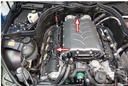
150 With the vacuum hose removed from the front of the factory manifold in step 52, loop the hose to connect each of end of the manifold runner activation solenoid.
