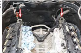
34 Reusing some of the T45 fasteners that mounted the lifting plate on the RH side of the engine, remount the transmission dipstick and wiring harness.
