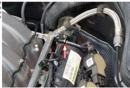
28 Disconnect the IAT sensor connector from the sensor, or remove the sensor from the manifold.
