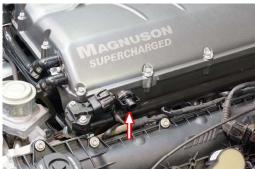
92 Connect the IAT extension harness to the IAT sensor and neatly route the IAT harness with the main injector harness.
