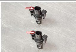
94 Install the factory MAP sensor with the supplied fasteners.
