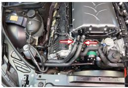
148 Route the throttle body extension harness along the right hand side of the motor.
