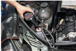
with the reservoir settled with as much coolant and water as possible, slowly release the bleeder screw to allow any air inside the LTR to escape. Once coolant and no air starts flowing, secure the bleeder screw.
