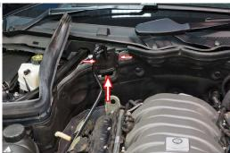
16 Compressing either side of the plastic locking ring, disconnect and remove the brake booster to manifold tube assembly.
