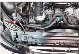
146 Install the supplied quick connect fittings to the colent manifolds and the cooler hoses. Check the orientation of the fittings once the hoses are pushed on as shown.
