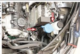
110 Using the supplied hose and clamps connect the purge hose to the purge solenoid as shown.
