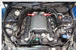
152 Install the new lower air boxes with the fasteners and washers supplied.
