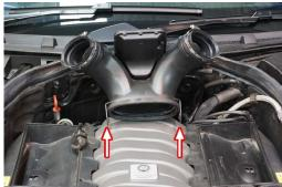
12 Remove the lower air boxes by firmly lifting and dislodging them from their mounting tabs in the shown locations.
