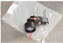
assembly to the engine and loosely torque the two (2) fasteners. Do not tension completely as this will be adjusted after fitting the supercharger.
