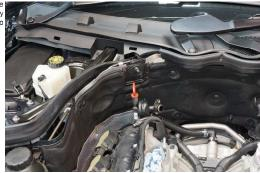
62 Ensure the cylinder head intake manifold faces are clean & free from debris, including all traces of original manifold gasket.
