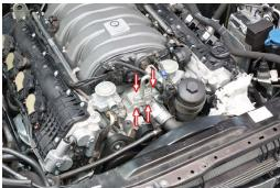
24 Disconnect the four (4) electrical connectors and the single vacuum line at the front of the manifold.
