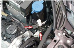
100 Gently pull the purge tube up over the washer bottle to allow access into the cavity behind the headlight.
