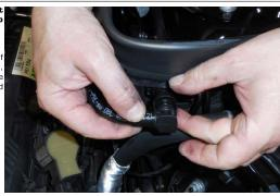
18 Disconnect the air valve hose as shown. If the vehicle has an electrical valve where the white joiner is shown, the valve stays on the long hose.
