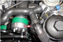
114 Using three (3) of the supplied short T25 screws, attach the degas reservoir mount to the bracket as shown.
