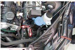
104 Install the supplied power steering return hose onto the new reservoir with the supplied clamp.
