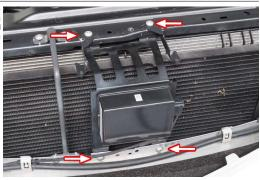
124Taking care not to damage the Low Temperature Radiator (LTR), temporarily lower it into position and mark the position of the top inlet as shown.
