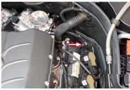
82 Trim the fuel emission hose to the appropriate length and clamp to purge tube as shown.
