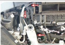
138 Remove the alternator terminal cap, remove the nut and route the pump harness power cable down and across to the terminal. Secure with the factory nut and reinstall the terminal cap.
