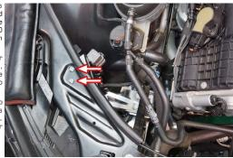
118 Install the earth wire of the Pump harness to the earth point on the RH side of the vehicle just beside the coolant reservoir as shown.
