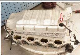
50 With the 2 throttle bodies revealed, remove both throttle body bell-mouths/ram-tubes (horizontal arrow), disconnect the breather lines (vertical down arrows) and disconnect the throttle body harnesses from the 2 throttle bodies (vertical up arrows).
