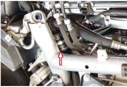
132Fit the supplied hose to the LTR. Clamp the short side to the LTR outlet as shown.
