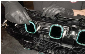
111. Remove intake gaskets from the OEM intake manifold. Inspect for damage, and replace as necessary. These will be reused.
