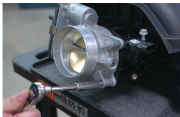
112. Remove the throttle body from the OEM intake manifold using a 10mm wrench. These four fasteners will not be reused.
