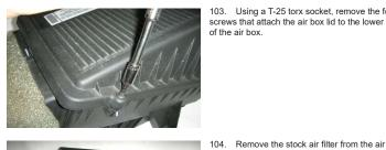
103. Using a T-25 torx socket, remove the four screws that attach the air box lid to the lower half of the air box.
