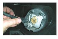
149. With the wheel well loose, pull back on the wheel well, giving you access to the fog lamps. Disconnect the electrical connector from the lamp. Repeat on the other side of the vehicle.
