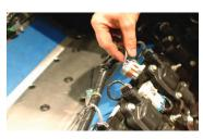
48. Reconnect the mail coil plug on both sides of the engine. NOTE: This ends the steps for 2011 and newer vehicles.
