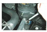
174. Now, put a piece of the remaining hose onto the other (lower) ½" barb on the intercooler reservoir and secure the clamp. Make sure you are using the supplied worm gear clamps.
