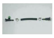
105. To create a new rear EVAP hose, cut a section of the 3/8"hose to 11" in length. Install the factory fittings removed in the previous step onto the ends.
