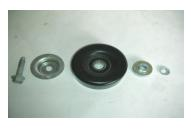
85. Using a soft hammer, knock the factory bolt loose from the idler pulley. The bolt retainer and stand-off pictured here on the right side of the pulley will not be re-used. NOTE: The bolt, dust cover and idler will mount to new tensioner bracket.
