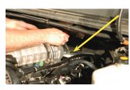
170. Starting at the intercooler barb on the driver side of the supercharger, attach the short end of the supplied 4 x 60 x 3/4"  $90^\circ$  molded hose with a #10 clamp. Run the hose forward and down beside the left side of the radiator.
