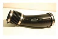
125. Assemble the bellows and coupler to the air tube. NOTE: The position of the clamp screws. The screws must be facing up so that you can install the assembly on the vehicle.
