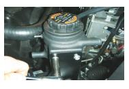
145. Mount the intercooler reservoir tank to the bracket using the three M6 X 12mm bolts. Tighten the bolts using a 10mm socket wrench.
