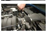
20. Pull up firmly on the air box assembly to separate from the three mounting grommet pins and remove from the vehicle.
