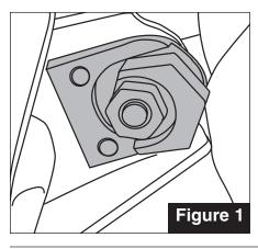
Caution: Do not try turning the cam in a full circle. Adjusting cam is not designed to rotate 360 degrees. Damage to the plate or cam may result.
