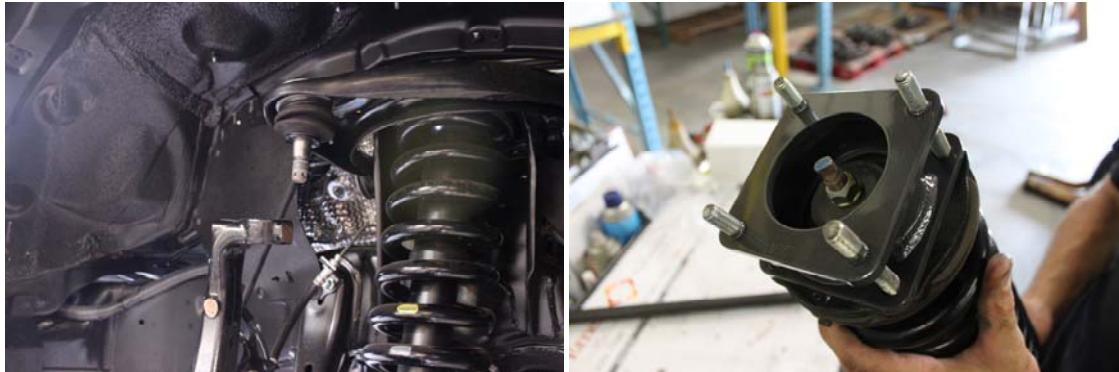
9. Reinstall strut into vehicle and install the new nuts provided, but do not tighten yet. Using a jack, raise the lower arm and guide both the lower strut mount and sway bar end link into their pockets. Install the lower strut mounting bolt and nut, torque to factory specs, use thread locker if necessary.
