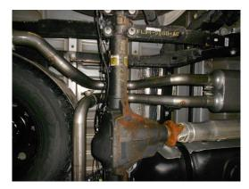
5) Install a provided clamp onto each of the muffler outlets. Then place the right side tailpipe **#86327S** into position over the axle and into the right side muffler outlet while also connecting the hanger on the pipe to the rubber mount on the vehicle. Tighten the band clamp enough to hold, but still allow for adjustment.
