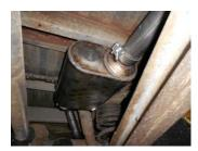
5) Take one of the **842548-Z** mufflers and place a supplied clamp onto the inlet, slide the inlet onto the back of one of the **86076S** inlet pipes with the outlet of the muffler in the center of the vehicle. Support the muffler with a stand and tighten the clamp enough to hold, but still allow for adjustment.
