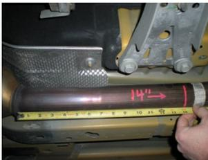
3) To install the new Flowmaster Scavenger X-pipe assembly **#16676S**, the factory Y-pipe must be removed. To do this, measure back 14.00" from the weld at the rear of each of the catalytic converters and make a mark on both pipes. Be sure to double check that the measurements are correct and cut both pipes on the marks. Remove any burrs.
