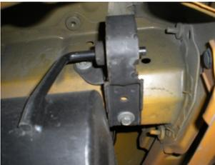
2) Unbolt the mounting brackets that mount the muffler to the frame (these are the two that connect the hangers on the *muffler body* to the frame). The mount connecting the hanger welded to the *inlet pipe* should remain bolted to the frame. Once these two hangers are unbolted, lower the muffler from the vehicle. Do not discard the OEM mounting brackets or hardware as they will be used in the installation of the new system. Lower the factory over-axle pipe from the vehicle and set aside.
