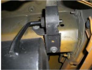
7) Install the OEM hanger bracket removed from the rear of the factory muffler **#852467-229**. Place the muffler up into position and connect the muffler inlet to the over-axle pipe. Bolt the hanger bracket to the frame using the OEM hardware. Connect the hanger on the front of the muffler to the factory mount on the vehicle.
