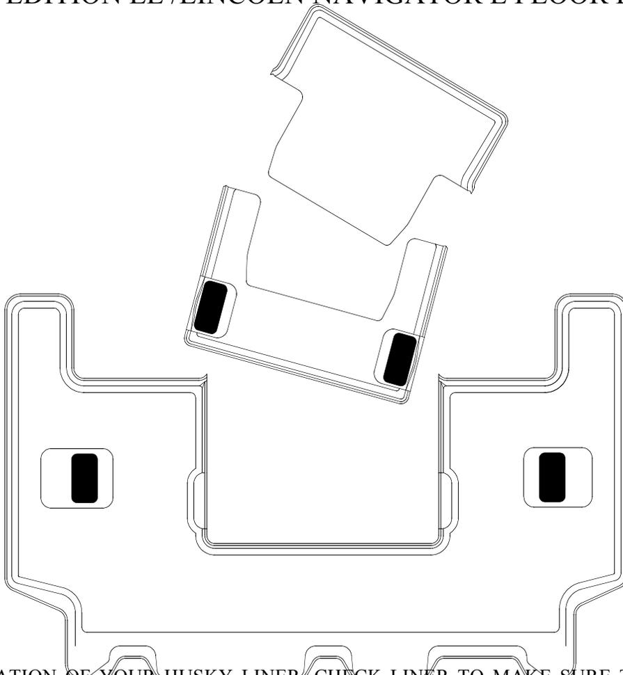
~~BEFORE INSTALLATION OF YOUR HUSKY LINER, CHECK LINER TO MAKE SURE THE FOUR (4) AREAS SHOWN ABOVE DARKENED ARE TRIMMED AWAY. IF THEY ARE NOT, DO NOT INSTALL LINER AS THE SECOND ROW OF SEATS WILL NOT LOCK SECURELY INTO POSITION. INSTEAD, PLEASE CALL HUSKY LINERS AT 800-344-8759.~~
