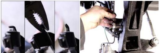
18. Remove stock brake line at the frame & caliper, then install new one. We suggest installing on frame side first, to let fluid bleed through the new line, then attach on caliper side.
