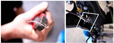
21. Remove the ABS line from behind the shock tower. Use supplied adell clamps to guide line across the Upper Control Arm, do the same with the clamps on the spindle using supplied bolts.
