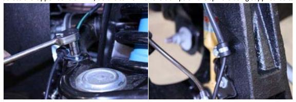
22. Tighten ABS sensor below the lower ball joint. Reinstall cotter pin to the upper ball joint and tie rod. See below for suggested brake line and ABS routing.
