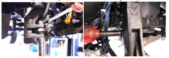
13. Rotate outer tie rods 180 degrees, this will now allow you to install the tie rod ends from the top of the steering arm.
