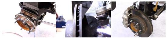
15. Remove the ABS line from the clip on the upper control arm, then remove the ABS line from the clip on the back of the shock tower.
