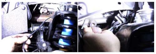
16. Remove bracket from upper control arm and discard, then remove ABS bracket from brake line bracket and discard
