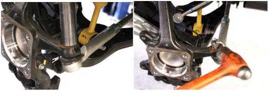
9. Remove the ABS Sensor, then upper ball joint nut.
