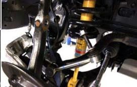
6. Remove the unit bearing, then discard backing plate & dust shield.
