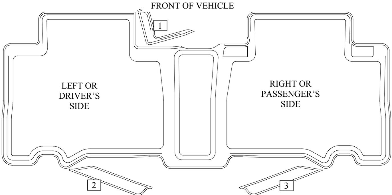
2006 RAV4 LIMITED MODELS WITH 3<sup>RD</sup> ROW SEATING HAVE CLIMATE CONTROL DUCTING ALONG THE REAR WALL OF THE 2<sup>ND</sup> ROW OF SEATS. THIS FEATURE KEEPS PART #6597 FROM FITTING CORRECTLY AS PACKAGED. HOWEVER, A TRIM AREA IS MOLDED INTO PART #6597 WHICH WILL ALLOW THIS PART TO BE TRIMMED TO ACCOMMODATE THE DUCTING. TO TRIM, REMOVE THE SECTION OF THE LINER SHOWN ABOVE (FIGURES #2 AND #3). USE THE FRONT EDGE OF THE RAISED BAND AS A TRIMMING GUIDE (SEE PHOTOS ON BACK).
