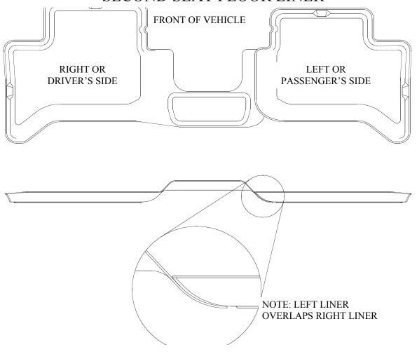
TO AID LINER INSTALLATION, MOVE THE FRONT SEATS TO THEIR MOST FORWARD POSITIONS. NOTE THAT THE PASSENGER SIDE LINER OVERLAPS THE DRIVER'S SIDE LINER.
