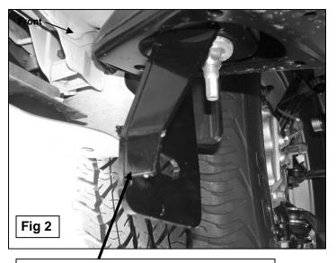
Install the front Mounting Bracket with the gusset toward the rear of the vehicle.
