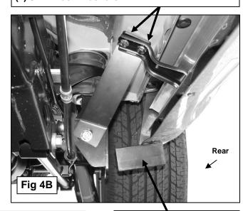
10mm x 25mm Hex Bolt (2) 10mm Flat Washers 10mm Lock Washer 10mm Hex Nut Remove plastic deflector.
