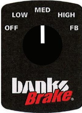
OFF mode allows the vehicle to behave as if the Banks Brake is not present.
