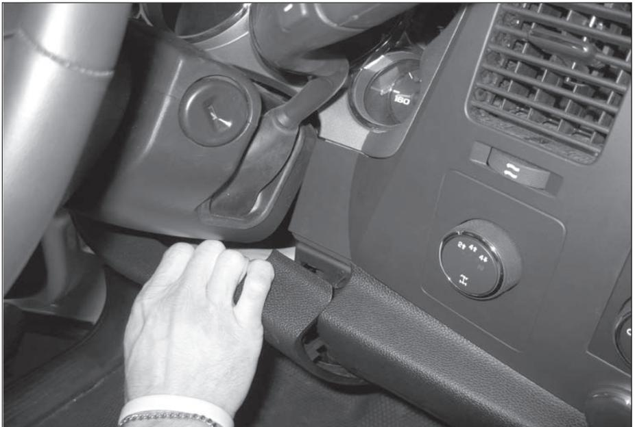
**16.** Under the steering column locate the 4-pin connection and disconnect. See **Figure 9**.
